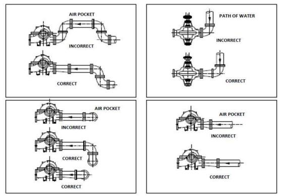
FIG. 4 SUCTION PIPING ARRANGEMENTS
