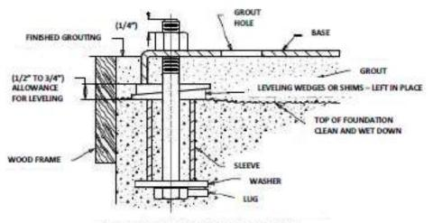
FIG. 3 TYPICAL FOUNDATION BOLT DESIGN
