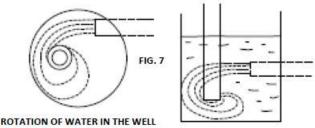
AS ILLUSTRATED CAN BE PREVENTED WITH A BAFFLE FIG. 7
