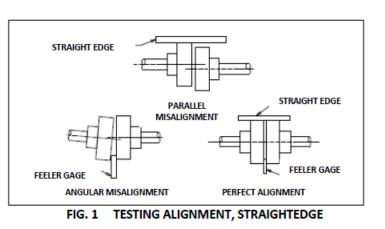
3. Check angular misalignment with a feeler gauge at four points 90° apart. Correct alignment occurs when the same gauge just enters between the halves at all four points.
